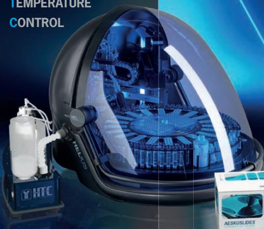
The **HELIOS®** Automated IFA System with the **HTC** Module sets and maintains optimal humidity point. The incubation takes place at up to 37°C. The built-in multi-type barcode reader is used for sample detection and identification. Sample-ring moves every 10 seconds during incubation to guarantee environmental homogeneity.
